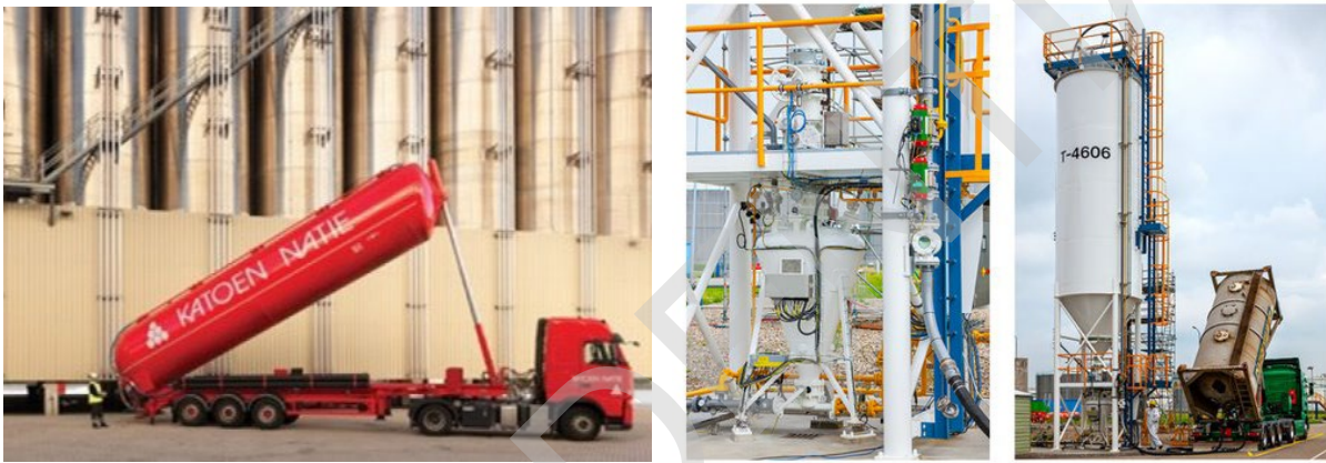
Figure 5 - Commercially available silo truck to transport metal fuels and storage silo's [Katoen Natie]
