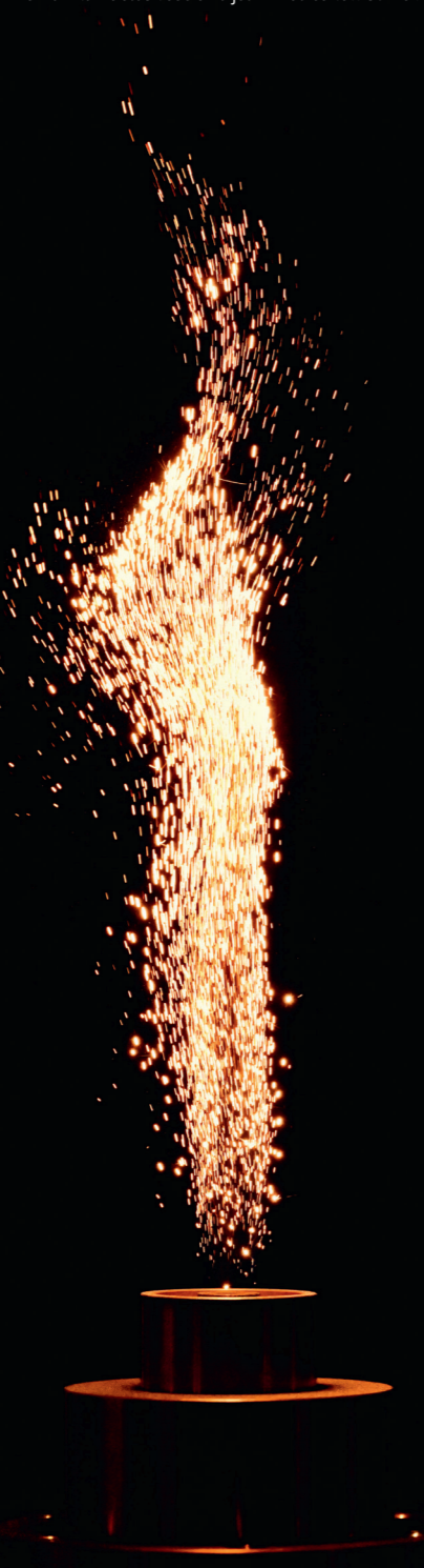
Iron-air flame stabilised on a jet-in-hot-coflow burner.
